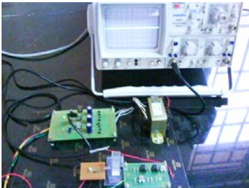
Fig. 11. Developed proto fluorescence sensing system showing deflection when arsenite solution placed in between transmitter and receiver circuit
