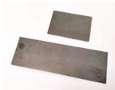
Fig. 2. The as-deposited \text{BiI}_3 thin film on glass substrates by ultrasonic spray deposition.
