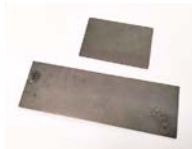
Fig. 2. The as-deposited BiI 3 thin film on glass substrates by ultrasonic spray deposition.
