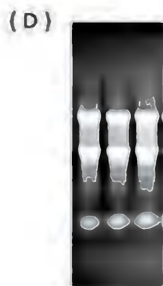
Fig.1D Formaldehyde-Agarose gel showing total RNA isolated from the fat body of last day fifth instar nymph.
